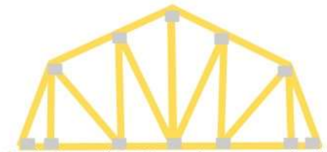
Gambrel Truss ( 2 different slopes to top chord)
